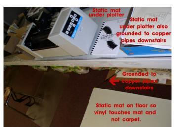
This photo shows the effective use of two anti-static mats in conjunction with a Gerber plotter. The customer who sent this picture to us has been thrilled with the results. Anti-static mats are easy to install and the benefits are immediate.
