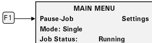
2. The current Job Status changes to **Paused**. To restart the job, press F1, Start-Job. The plotter returns to the previous position and resumes cutting or plotting.
