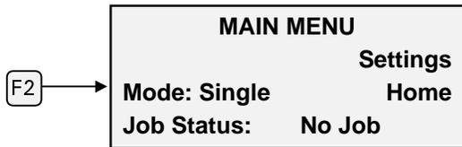
2. Send the job to the plotter. When the job reaches the plotter, the status changes from **No Job** to **Ready**, and **Start-Job** blinks (indicated by the dotted box around Start-Job in the diagram below).
