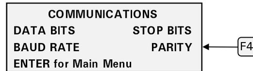
11. Press F3 and F4 to change Parity. You can choose **none**, **even**, or **odd**. Press ENTER to accept the new setting and return to the Communications menu.
