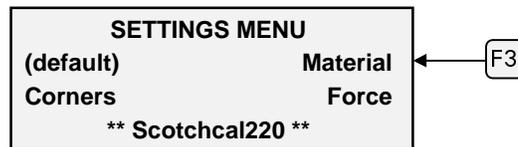
2. Use F3 or F4 to toggle up or down through the list of materials. Select the one you are using by pressing ENTER. (See “Fine tuning the enVision” on the next page for more information on using this screen to fine tune your plotter to the job.)
