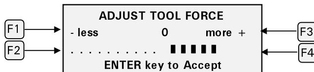
Pressing the F1 (or F2) key would cause the bar graph to move in the opposite direction, retracting toward the zero point one click for each press. When it reaches the zero point, the factory default has been reset. Continued pressing of the F1 or F2 key will extend the bar graph to the left of the zero point and reduce the factory default by the number of clicks that F1 is pressed.
