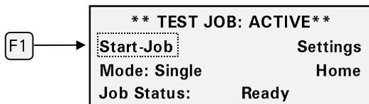
The plotter generates the X08 test pattern. If the plotter is in Single mode, as above, it will stop when one test pattern has been cut. If it is in Multi mode, it will continue to cut one test pattern after another until you press CANCEL to stop it. Compare the test cut to the illustration on the previous page.
