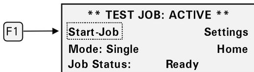
The plotter generates the Wagon Wheel test plot. If the plotter is in Single mode, as above, it will stop when one test pattern has been plotted. If it is in Multi mode, it will continue to plot one test pattern after another until you press CANCEL to stop it or switch back to single. Compare the test plot to the illustration on the previous page.
