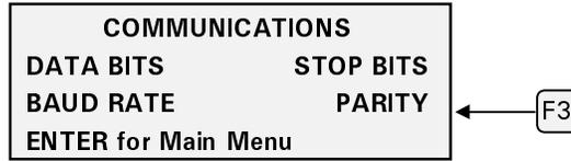
9. Press F3 and F4 to change the number of Stop bits. You can choose between 1, 1.5, and 2. Press ENTER to record setting and return to the Communications menu.
